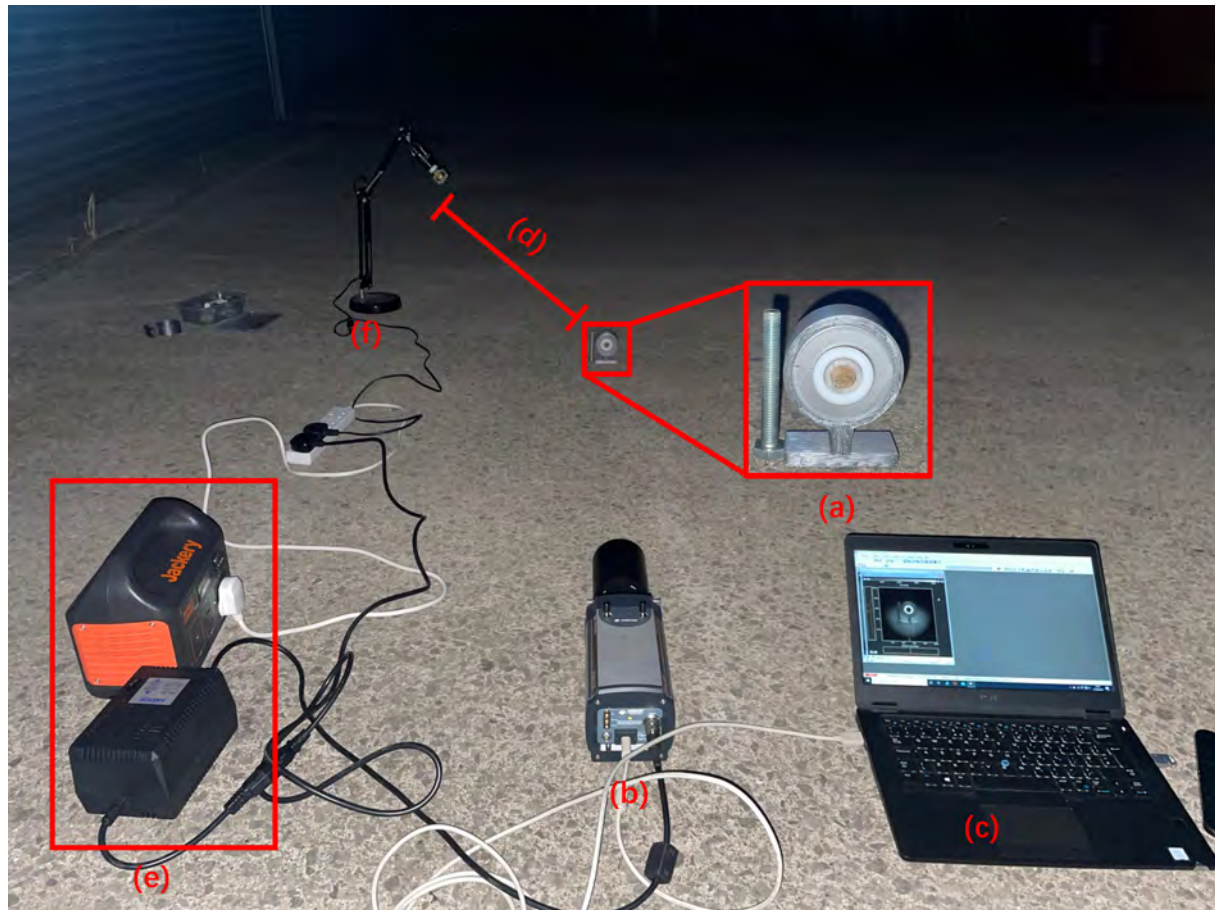
Figure 7. Experimental setup for night-time imaging of alpha RL: (a) alpha source, (b) alpha camera, (c) controlling laptop, (d) distance between light bulb and alpha source, (e) power bank and supply, (f) light lamp simulating ambient light source.
